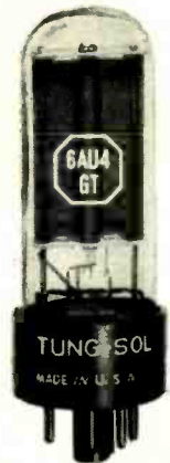
Below—New Tung-Sol 6AU4-GT damper diode is designed for 90° deflection systems.
