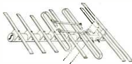
Fig. 11—Mechanical arrangement of Snyder u.h.f. broad-band Yagi. Note that reflectors are mounted one above the other, and lead-in goes to front dipole.
