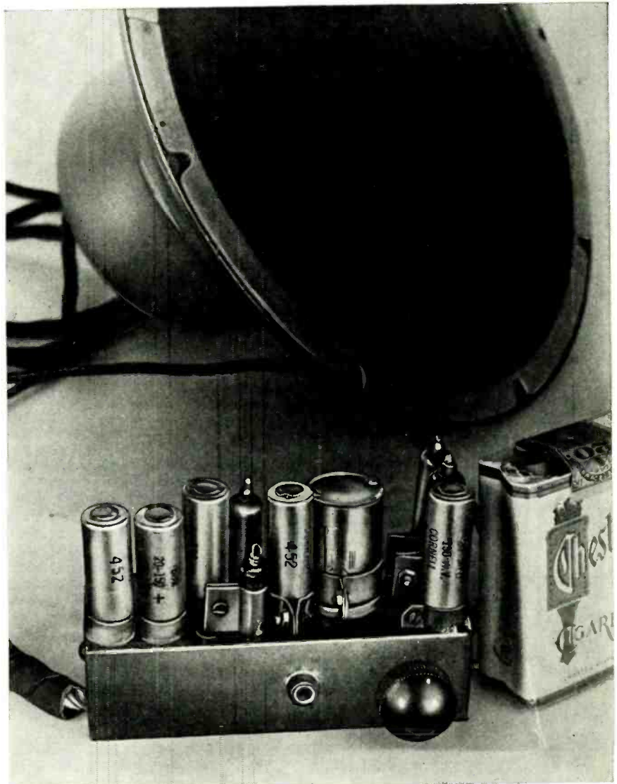
This 3-watt a.f. amplifier is pocket size. Special miniature parts are used.
