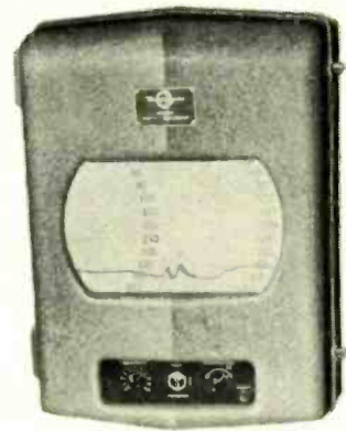
Fig. 4—Bendix recording-type depth indicator maps seabed contour down to 400 fathoms on a roll chart. Switch in center converts indications to feet.
