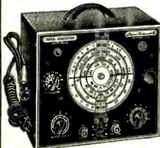
• Tubes used: 1-6BE6 as R. F. Oscillator, mixer and amplifier. 1-6BE6 as Audio Oscillator. 1-6X6 as Power Rectifier.
